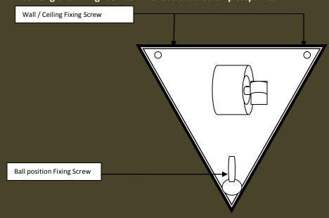
Step 2: Insert ball component in the mounting component
